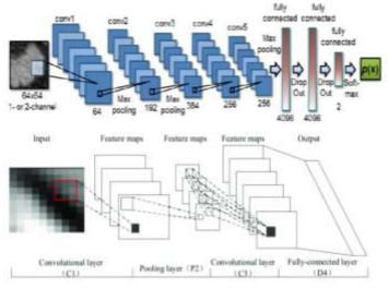
Figure 4: CNN Architecture
