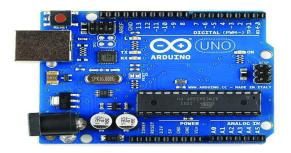
FIG: Arduino Uno Board
