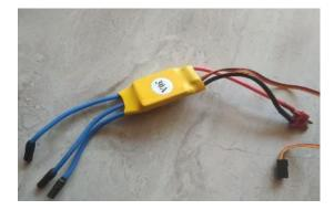
FIG: ESC (Electronic Speed Controller)
