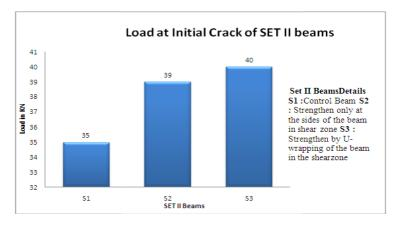
Fig. 3: Load at initial crack of beams S1, S2 and S3.
