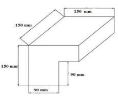
Figure.4: Shear plane 150\*60 mm
