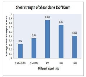
Figure.7: The variation of shear strength test results (shear plane 150\*80)
