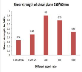
Figure.9: The variation of shear strength test results (shear plane 150\*60)
