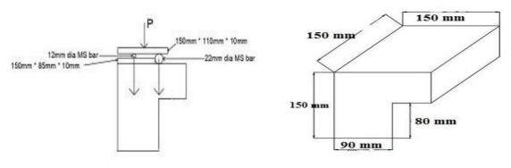
Figure.1: Shear strength test setup
