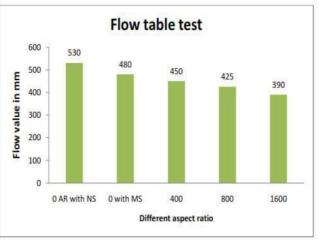
Figure.11: The variation of flow table test results
