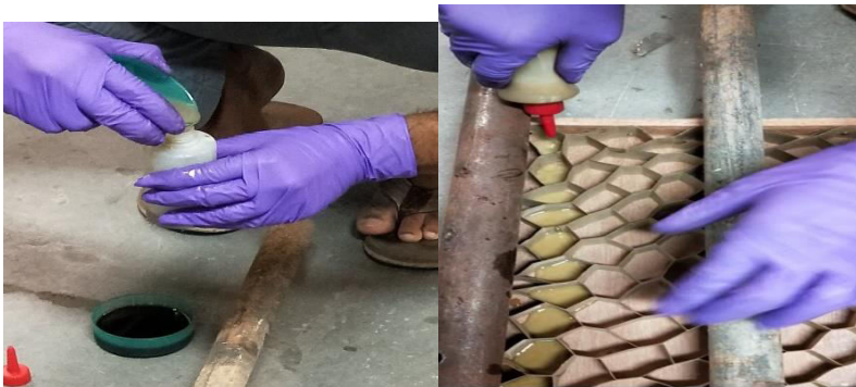
Fig: 8 Mixing Of Polyol and isocyanate
