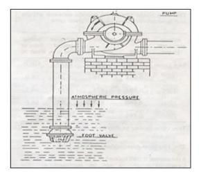
Fig. 6:Priming by foot valve
