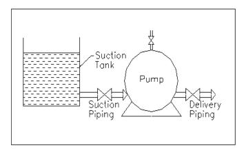
Fig.3:Priming with flooded suction
