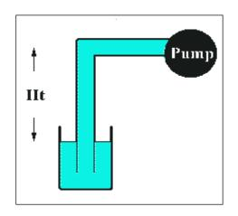
Fig.2: Priming principle
