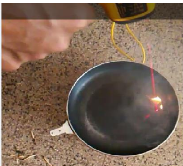
Fig -4: Spark of the Flash Point Testing
