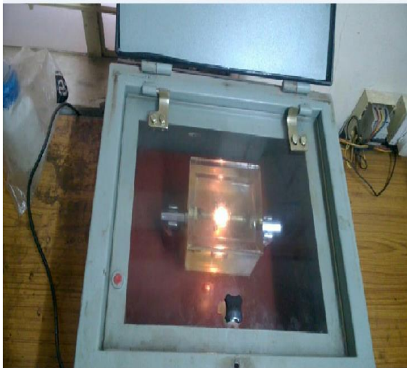
Fig -3: Spark of the break down voltage
