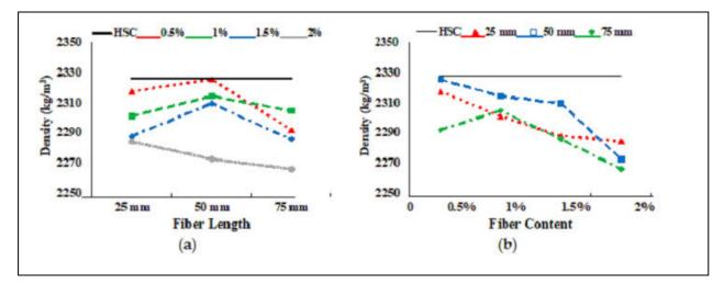
Figure: Influence on density: (a) Fiber length; (b) Fiber content.
