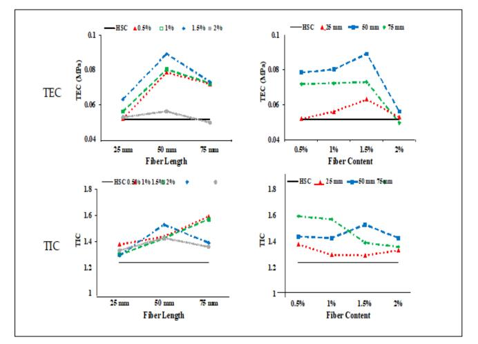
Figure :- Influence of coconut fiber on PEC, CEC, TEC, and TIC: (a) Length; (b) Content.
