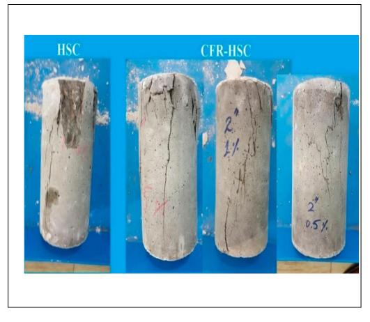
Figure: (b) HSC and CFR-HSC specimens after compressive strength tests.
