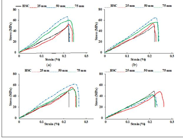
Figure: (a) Stress-strain curves for HSC and CFR-HSC with (a) 0.5%, (b) 1%, (c) 1.5%, and (d) 2% fiber content.
