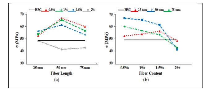
**Figure:** Influence on  $\sigma$ : (a) Fiber length; (b) Fiber content.
