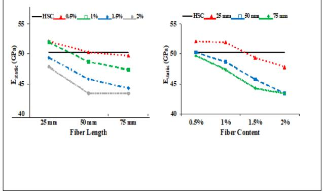
Figure: Influence on  $E_{static}$ : (a) Fiber length; (b) Fiber content
