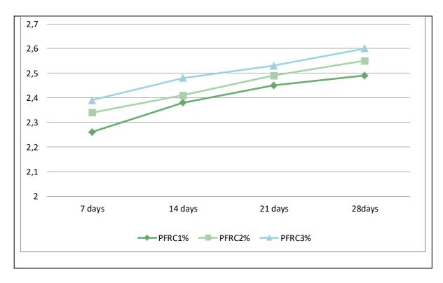
Figure: (b) compression of compressive strength m-30 PFRC & conventional concrete of PFRC1%, PFRC2% & PFRC3%.
