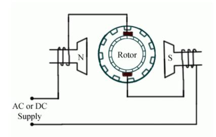
Fig.2 Mixer Grinder Circuit
