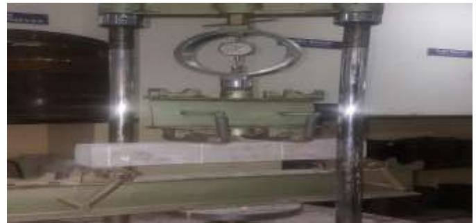
2.11 Specimen for flexural strength testing
