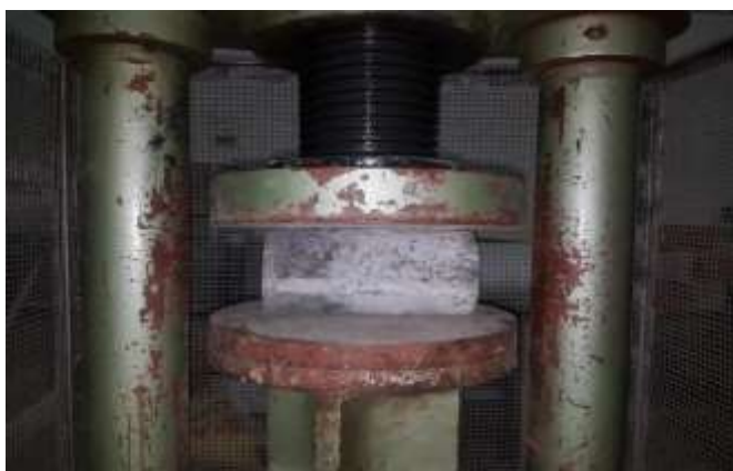
Figure 2.10 Specimen for split tensile testing
