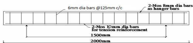
Fig.3.8 (b) Longitudinal Section of Beam
