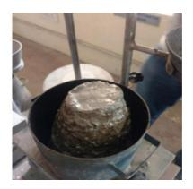
Figure 4.1- (a) Slump test (b) Vee Bee test
