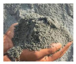
Figure 3.2- Sample of M-sand material
