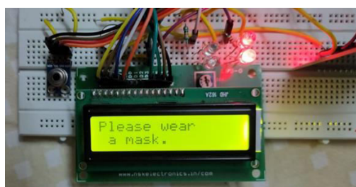
Figure 14: LCD Display and LED Output for not wearing a mask
