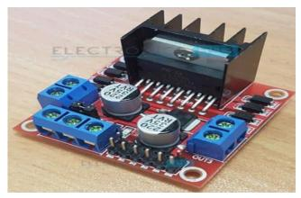
Fig -3: L298 Motor Driver Module
