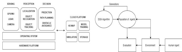
Fig. 3.2 Existing system architecture used for autonomous driving technologies [6]
