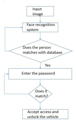
Fig 2: System flow diagram
