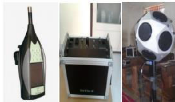
(a) Bruel and kjaer (BK 2250) sound level meter used for measuring Reverberation time. (b) 2734-B power amplifier. (c) 4292-L Omni Power sound source.
