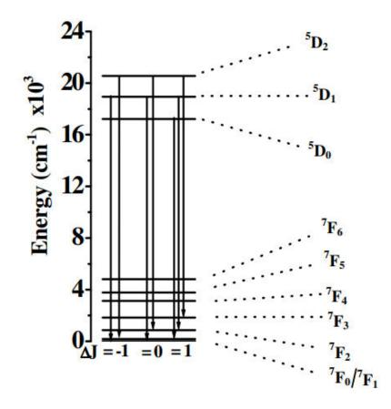
Fig.1.6. Energy level diagram of Eu<sup>3+</sup> in nanocrystalline Y<sub>2</sub>O<sub>3</sub>:Eu<sup>3+</sup>
