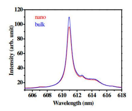
Fig. 1.8 Emission spectrum of 612 nm line for nanocrystalline and bulk phosphors
