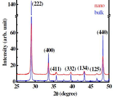
Fig. 1.3. XRD pattern for nanocrystalline and bulk phosphor
