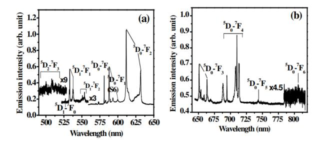
Fig. 1.5. Emission spectrum of nanocrystalline  $Y_2O_3$ : Eu<sup>3+</sup> for  $\lambda_{exc} = 488$  nm. Intensities of (a) and (b) are not in the same scale.
