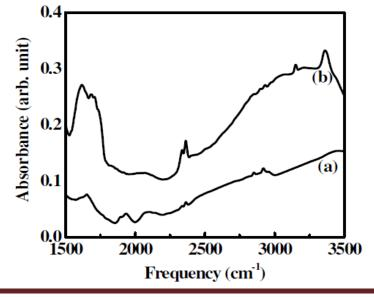
Fig.1.2. FTIR spectra of (a) TEA (Triethanol amine) without heat treatment and (b) Solution of TEA complexed with metal ion just before decomposition.
