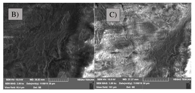
Fig 4: SEM photography of CuO nanoparticle and CuO/ PVA thin film.
