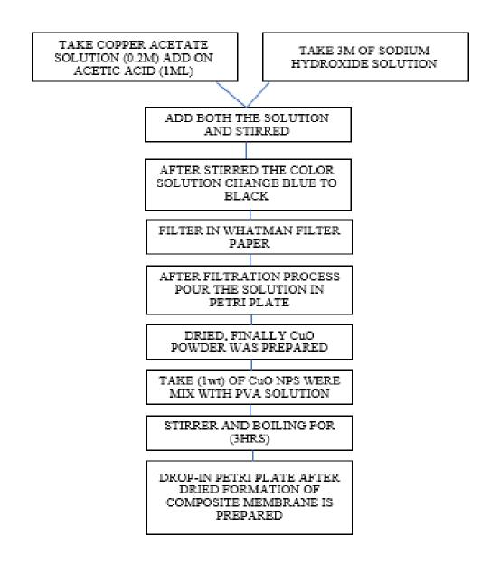
Fig 1:This flow chart represents the synthesis process of CuO/PVA thin film.
