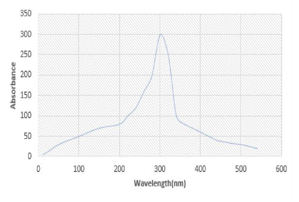
Fig 3: uv-spectroscopy of CuO/PVA solution.
