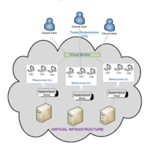
Fig. Management system of task scheduling and resource allocation.
