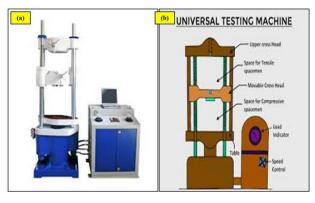
Fig 5. (a) Universal Testing Machine (b) UTM Line Diagram
