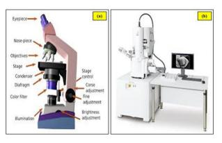
Fig 4. (a) Optical Microscope (b) Scanning Electron Microscope
