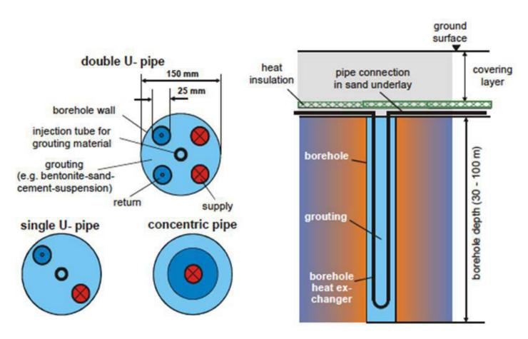
Figure 4 Types of borehole heat exchangers [14]
