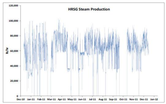
Figure 8 Hourly steam produced by the HRSG
