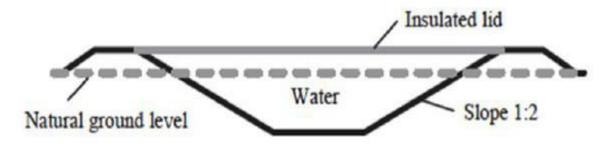
Figure 3 Cross section of the PTES [15]
