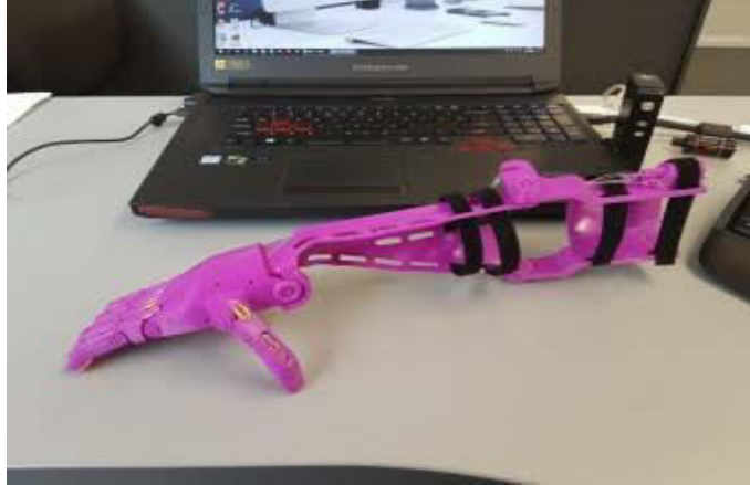
Figure 6 Prosthetic arm made of PLA
