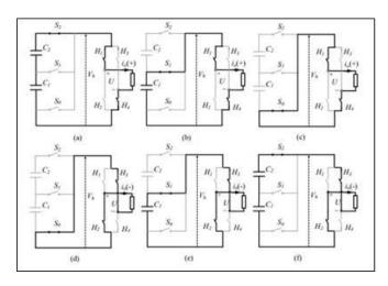
Fig 2. Working Mode of Multi-Level Inverter
