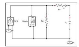
Fig 4. Schematic Diagram for Solar PV system
