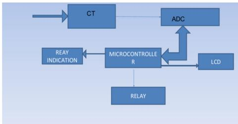
1. Analog signal (current) is obtained from the transmission line and is reduced by the current transformer.
