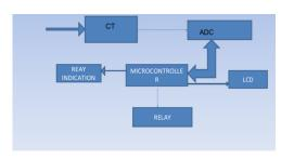
1. Analog signal (current) is obtained from the transmission line and is reduced by the current transformer.
