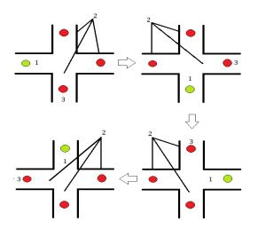
In this diagram, green denotes the side/lane with green signal on and red denotes the remaining sides with red signal on. Following diagram depicts the one complete iteration of traffic signal.
