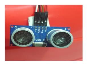
The Sonic Sensor is used for computing the depth. Here it is used to measure the depth of the septic tank. The Sonic Sensor is fixed into the Septic tank. Then the Septic tank get filled means, it can sends the communications to particular organization. Then they will allot persons to clean the septic tank. Then septic tank cleaners will clean the tank. After cleaning it, the sensor can detect the level, and send messages to
