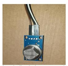
It cansintellect the dry gases present in the toilets such as NH3, CO2, CH4, H2S, etc. By taking thosegases leads to Nausea, Drowsiness, instant loss of awareness, etc. After sensing the unwanted gases, it can blink the red light. Then the sweeper can clean it by using particular Cleaning Agents.
