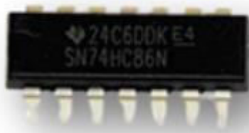
Fig. 6. EX-OR Gate (IC 7486)
