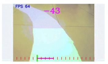
Figure 13: Real time detection of lane with curve value
