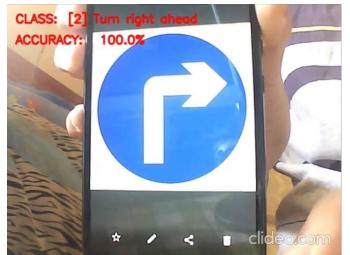
Figure 15: Real time recognition of turn right ahead sign
