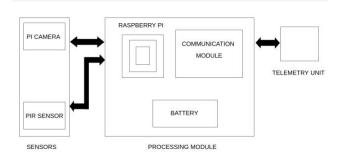
Fig 2. Block Diagram of Image Processing Module
