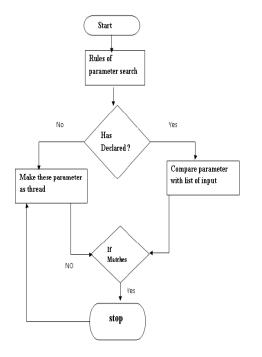
The whitelist filter algorithm checking multiple things. First Whitelist filter checks if the parameter is declared in list . Then whitelist applied on every parameter . If the parameter not matched then whitelist filter restricted this parameter. If parameter matched then it passed this parameter.
