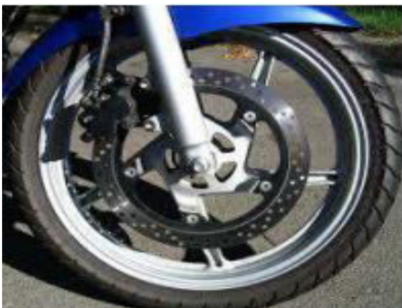
Figure 1: Disc brake assembly mounted on front wheel [1]
