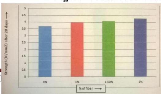
**Figure 8: Result of flexural strength Test after 28 Days**
