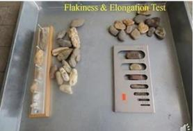
Fig. 3 Flakiness and Elongation Test Apparatus
