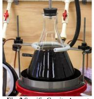
Fig. 2 Specific Gravity Apparatus
