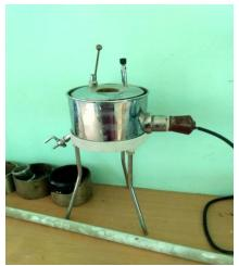
Fig. 1 Standard Viscometer
