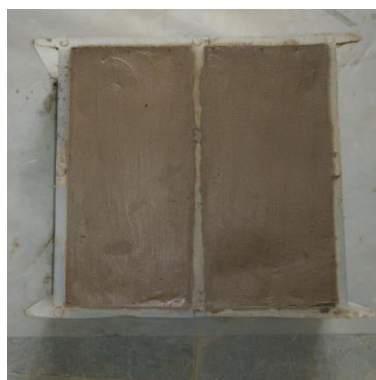
Fig 2 Casting of bricks 3
