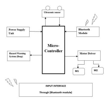
Fig 1.1 Vehicle Collision Avoidance System Architecture diagram
