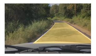
Figure 8. Lane detection using CNN.
