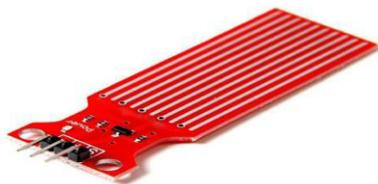
**Fig -4: Water Level Sensor**
