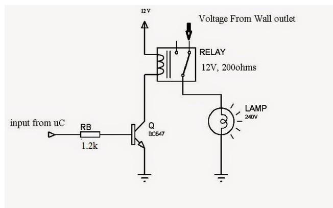
**Fig -7: Relay Driver Circuit**
