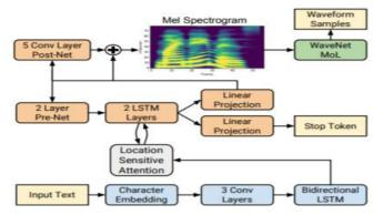
Figure 3.4 - Tacotron-2 Architecture
