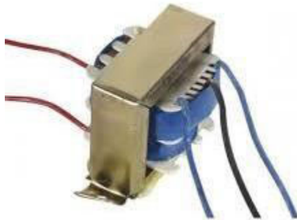
Fig -1: Step Down Transformer
