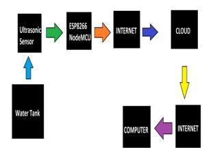
**3.1Ultrasonic Sensor** :An ultrasonic sensor transmits ultrasonic waves into the air and detects reflected waves from an object. There are many applications for ultrasonic sensors, such as in intruder alarm systems, automatic door openers and backupautomobile The ultrasonic sensor works on following formula
