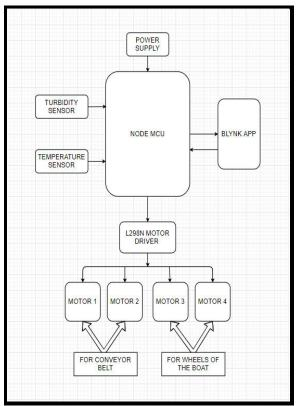
Fig-1: Block Diagram of WQMC
