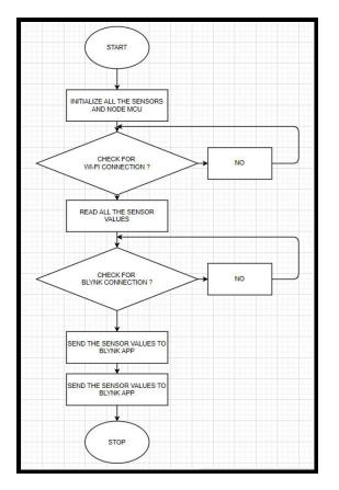
Fig-2: Flowchart for Water Quality Monitoring
