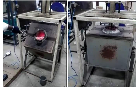
Fig.2 Stir Casting Process
