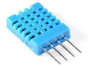
DHT11 Humidity Sensor consists of 4 pins: VCC, Data Out, Not Connected (NC) and GND. The range of voltage for VCC pin is 3.5V to 5.5V. A 5V supply would do fine. The data from the Data Out pin is a serial digital data
