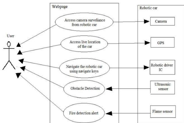
Figure 1: Block Diagram of actual working
