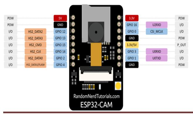
The ESP32 CAM WIFI Module Bluetooth with OV2640 Camera Module 2MP For Face Recognition has a very competitive small-size camera module that can operate independently as a minimum system with a footprint of only 40 x 27 mm; a deep sleep current of up to 6mA and is widely used in various IoT applications.
