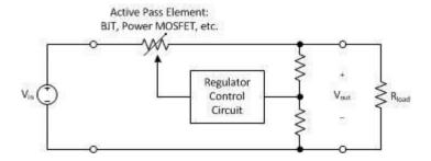
The pass element functioning as a variable resistor can be semiconductor devices such as a bipolar junction transistor (BJT), power metal oxide semiconductor field effect transistor (MOSFET), insulated gate bipolar transistor (IGBT), or an electron tube such as a triode, tetrad, or pentode. Electron tubes would be used in highly specialized applications where there are no semiconductor devices suitable.
