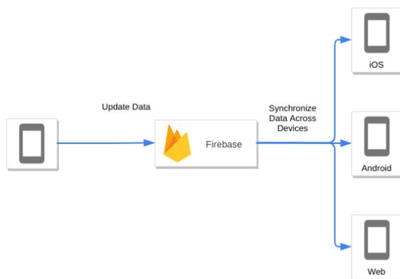
Realtime Database (RTDB) stores the data as JSON tree. It offers many client SDKs from iOS, Android, and Web. The database of the system consist of three Schemas – one that holds the information about the user which consist of fields like email id, user name, authentication details, gender etc, another one stores the data about the roads, their addresses, the ratings and the last one consist of the data about the contractors and the rating calculated from the second table.
