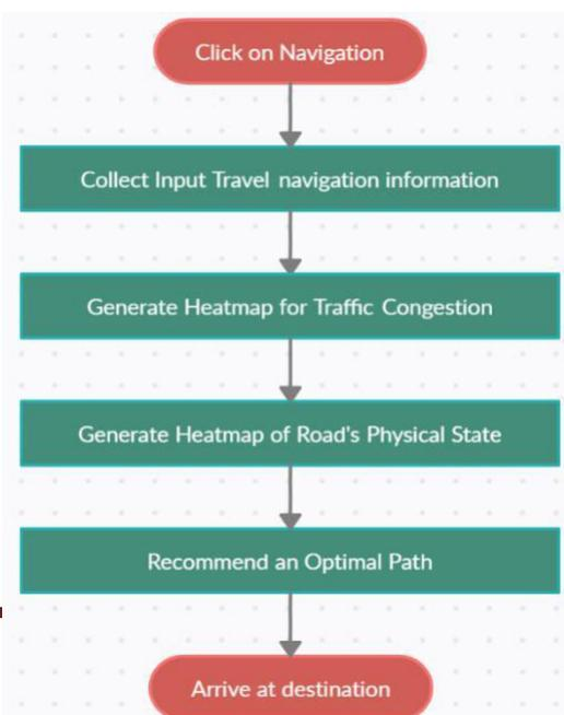
congestion of traffic vehicles, the system generates another heat for physical state of the road and allows user to optimize the route according to time takes in order to cross a nicely paved road vs a damaged road.
