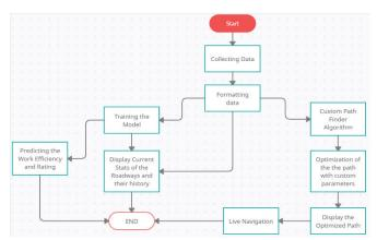
Prediction of state of the road is very challenging and complicated process because it depends on multiple factors and is time varying. The factors being the weather conditions, the movement of heavy vehicles etc. Although the life of road is pre-decided at the time of estimation, it erodes way before the lifetime speculated earlier. We will be using Random Forest algorithm in order to combine these factors together to train the prediction model.
