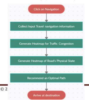
congestion of traffic vehicles, the system generates another heat for physical state of the road and allows user to optimize the route according to time takes in order to cross a nicely paved road vs a damaged road.
