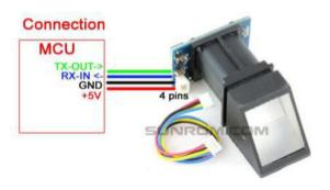
Figure 2: fingerprint sensor
