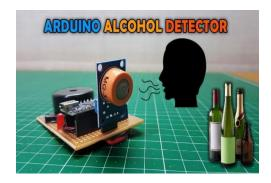
Here we check the alcohol level of driver. If the driver drunk the alcohol, vehicle doesn't start. Buzzer will produce the sound.
